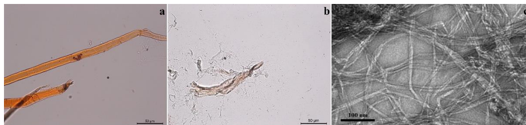
Fig. 2 Light microscopy (LM) images of the fibers:(a) before defibrillation; (b) after defibrillation; (c) Transmission electron microscopy (TEM) micrograph of the nanofibrils from the defibrillation process
